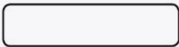
The solid-edge profile is ideal when board edges are visible, such as picture-frame boards or stair treads. Solid deck boards should be fastened through the top of the board using composite deck screws.
