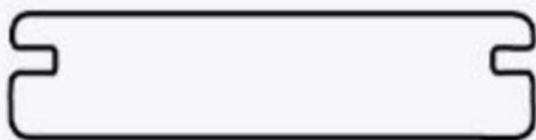
Grooved-edge decking gives a clean, fastener-free appearance to the surface of your Deckorators deck. Stowaway™ hidden fasteners are a perfect way to discreetly secure deck boards to joists using the grooved edges.
